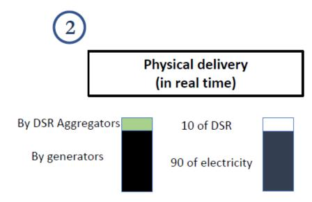
Actual consumption (90) (as reduced by DSR) is balanced by actual electricity generation (90)
