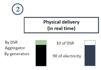
Actual consumption (90) (as reduced by DSR) is balanced by actual electricity generation (90)
