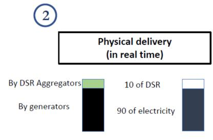
Actual consumption (90) (as reduced by DSR) is balanced by actual electricity generation (90)
