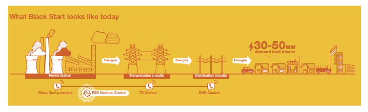
An **LJRP** is used to form a Power Island. As the restoration progresses, individual Power Islands are subsequently connected together to form wider Power Islands. This facilitates the connection of other parties including Generators and Embedded Generators without any current restoration capability.
