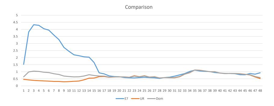
The load shapes for E7 and UR look different as expected. The Domestic shape reflects both the E7 storage load and the UR night load shape. If volumes were separately applied to the UR and E7 shapes the outturn 'Super Customer' load shape used in imbalance settlement would look like the domestic shape above.
