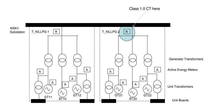
Active Metering only – Compensated for VT & CT Errors and Transformer losses
