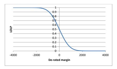
From the graph above it is clear that at 0MW of de-rated margin (note that at this point the only margin remaining is reserve for response which cannot be depleted) the LoLP value is 0.5. This is because when there is expected to be no de-rated margin available at Gate Closure there is statistically a 50:50 chance that there will be sufficient generation during the Settlement Period to meet demand i.e. because demand could reduce or generation increase or vice versa.
