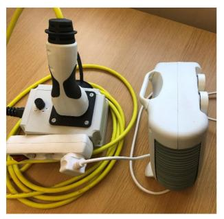
The load is measured via a separate MID approved meter, unrelated to the equipment.
